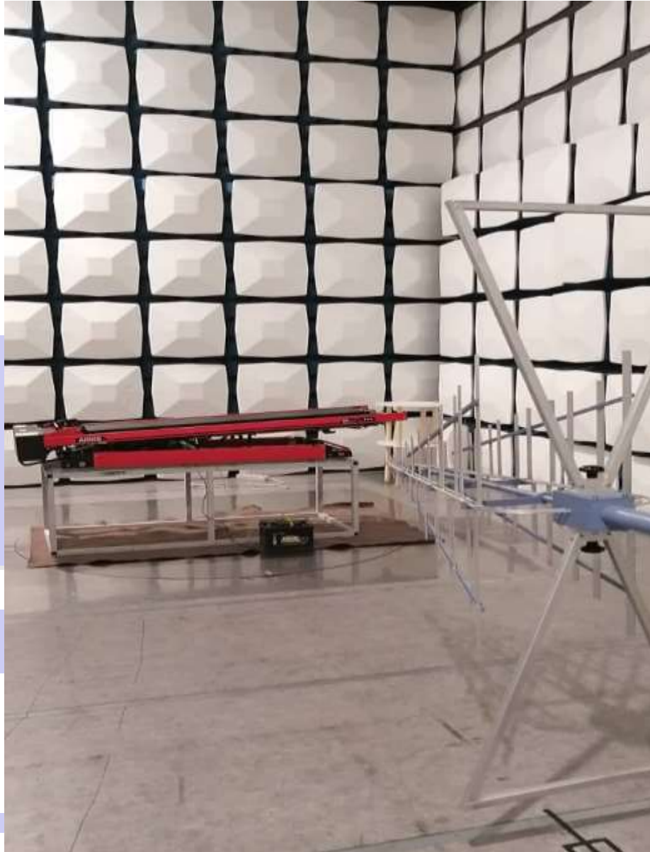
Figure 6: Equipment under Radiated Emission Test
